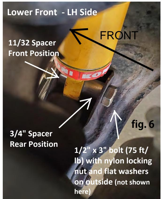
14. On the front control arms, drill out the lower shock bolt tabs to 1/2" diameter. -- fig.6
