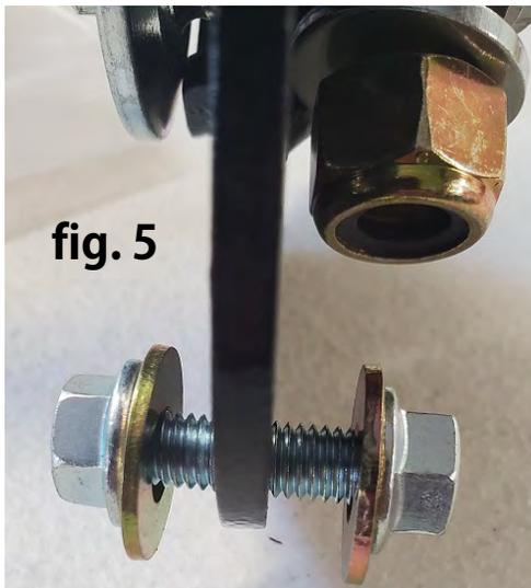
Install M8 hardware on upper mounts as shown
